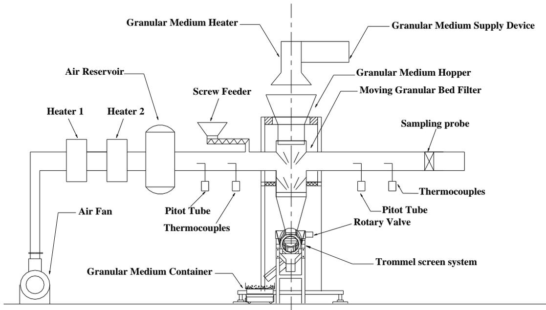
**Fig. 1.** Schematic diagram of the current experimental moving granular bed filter (MGBF) apparatus.
