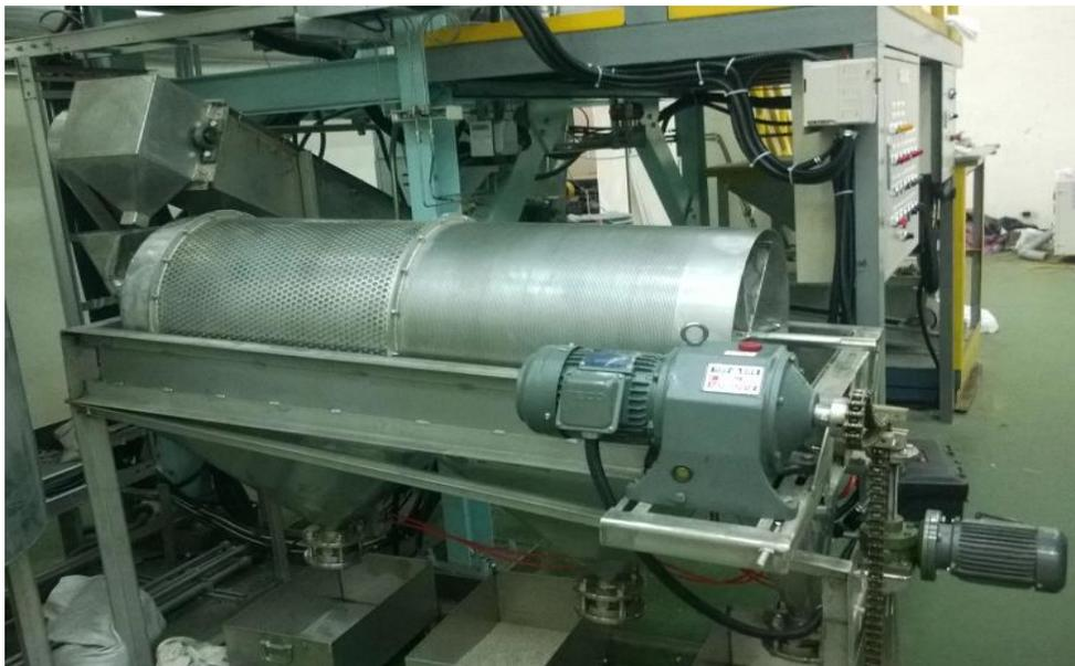
**Fig. 2.** Trommel screen system
