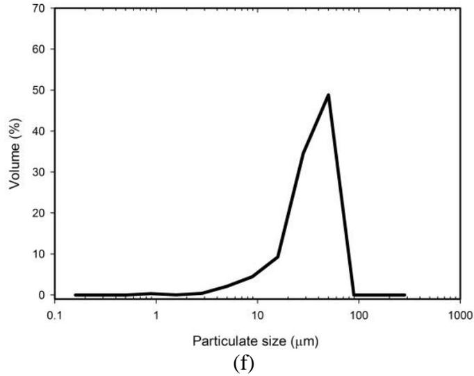
**Fig. 5.** Size distribution of the dust particulate exiting the moving granular bed filter bed for operation temperatures of: (a) 20 °C, (b) 100 °C, (c) 200 °C, (d) 300 °C, (e) 400 °C, and (f) 500 °C, with a fixed filtration superficial velocity of 35 cm/sec and mass flow rate of 600 g/min.
