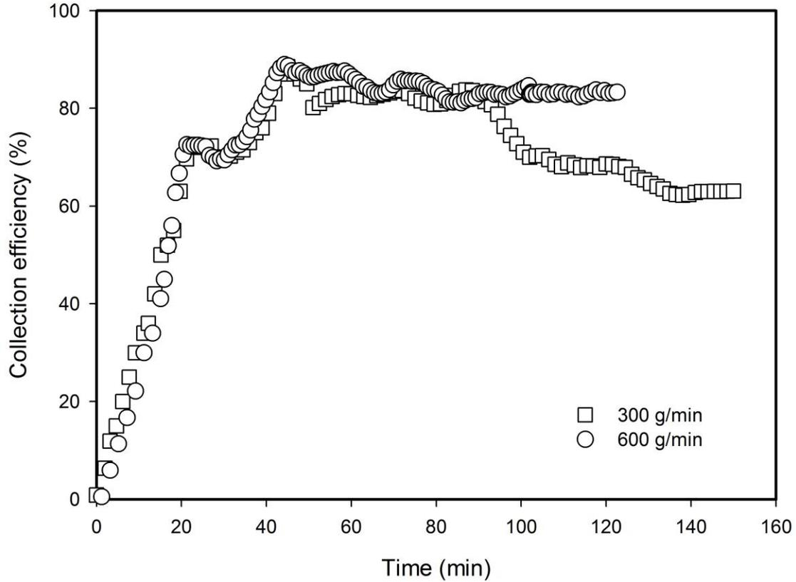
**Fig. 3.** Variation of the collection efficiency with filtration time for different mass flow rates of 300 and 600 g/min, with the fixed filtration superficial velocity of 35 g/min and room temperature of 500 °C.
