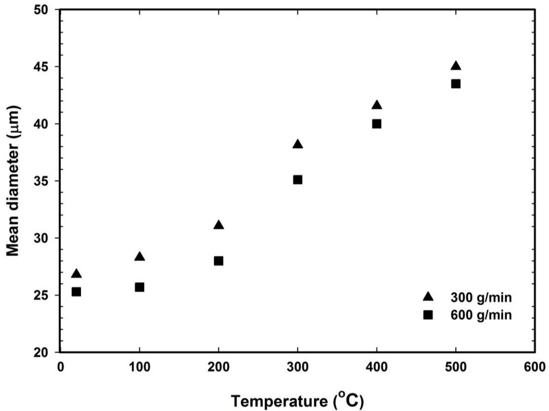
**Fig. 6.** Mean diameter of the dust particulate at outlet filter system under various operating conditions.
