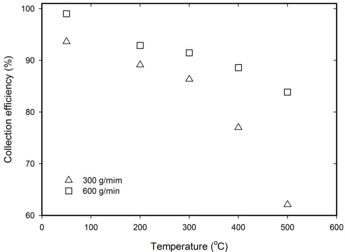
**Fig. 4.** Variation of the collection efficiency with different operation temperature and mass flow rate, with the fixed filtration superficial velocity of 35 cm/sec.
